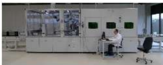
Automated module manufacturing for new technologies, full-size modules Pick & place, dispensing, lasering, soldering
